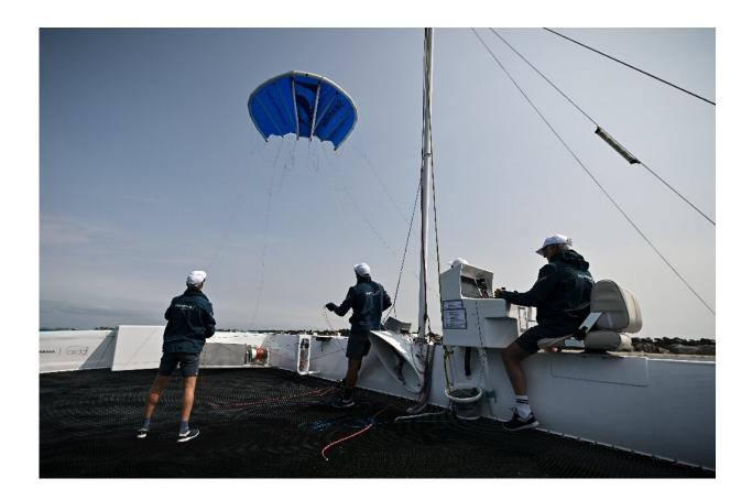
The startup Beyond The Sea tests a blue inflatable kite sail the size of a small studio to pull a specially-designed catamaran across the water.
