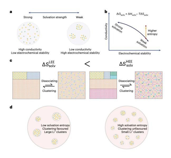
Design framework for HEEs. a, Schematic illustrating the apparent trade-off between ionic conductivity and electrochemical stability in tuning the solvation
