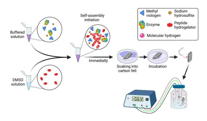
Schematic diagram of electrode preparation. Credit: *Carbon Energy* (2023). DOI: 10.1002/cey2.411
