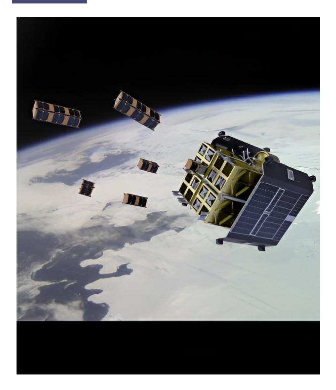
The ION SCV004 satellite, on which the machine learning models were run. The image shows the satellite releasing CubeSats (small satellites) into space. Credit: D-Orbit
