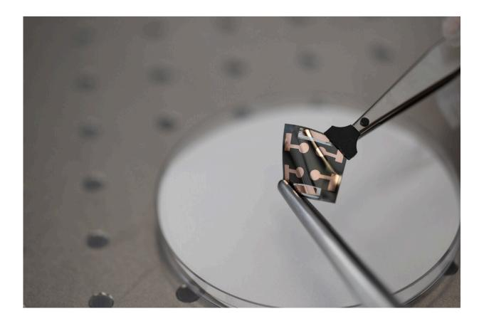
A perovskite solar cell is examined using laboratory equipment. Credit: The University of Sydney
