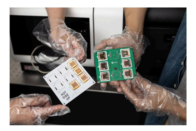
Anita Ho-Baillie and Shi Tang wear protective gloves while examining perovskite solar cell prototypes. Credit: University of Sydney
