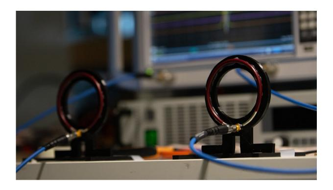
Two loop antennas (radius: 3.6 centimeters) can transfer power between each other from 18 centimeters apart. Credit: Nam Ha-Van/Aalto University
