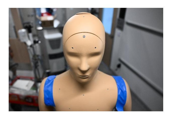
Pores that bead sweat like humans are displayed on ANDI, an Advanced Newton Dynamic Instrument, as researchers prepare to learn more about the effect of heat exposure on the human body at Arizona State University (ASU) on July 20, 2023.
