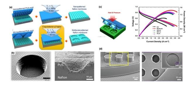
Designing polymeric membranes using imprinting technology to improve fuel cell performance. Credit: Korea Institute of Science and Technology
