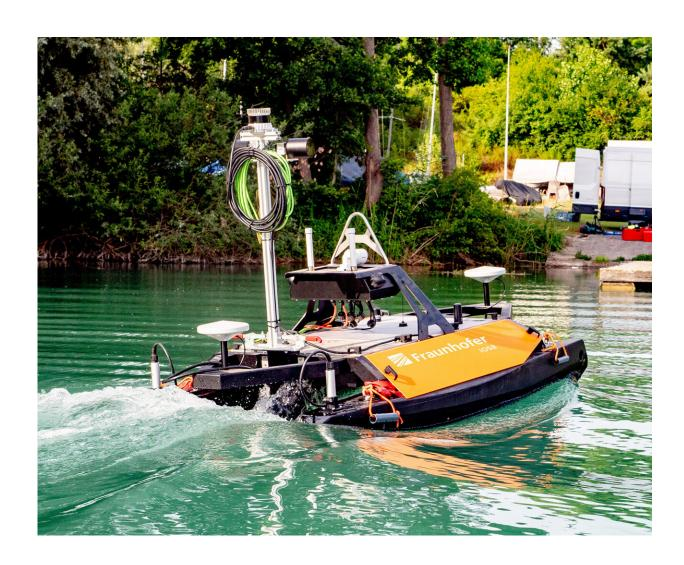
The USV in action, using the autonomous capabilities and sensors for underwater and above-water mapping fitted as part of the TAPS project. Credit: © Fraunhofer IOSB
