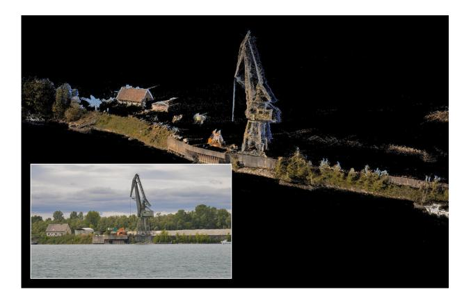
Three-dimensional reconstruction of the bank structures generated by combining the cameras and laser scanner—and, for comparison, a photo of the same section of bank taken from the perspective of the watercraft. Credit: Fraunhofer IOSB
