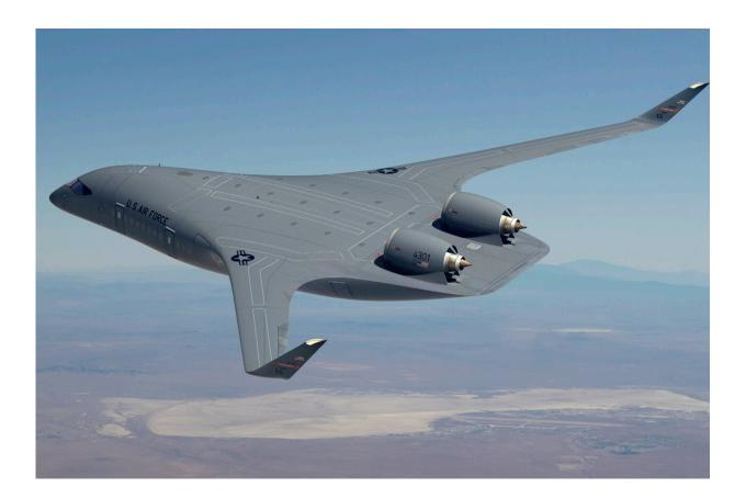
This image provided by the U.S. Air Force shows a rendering of a blended-wing body prototype aircraft. The Air Force has promised \$235 million to help startup manufacturer JetZero build a jet with a blended-wing body that officials say could provide greater range and efficiency for military tankers and cargo planes and perhaps eventually be used to carry airline passengers. JetZero and the Air Force, which announced the award Wednesday, Aug. 16, 2023, say they hope
