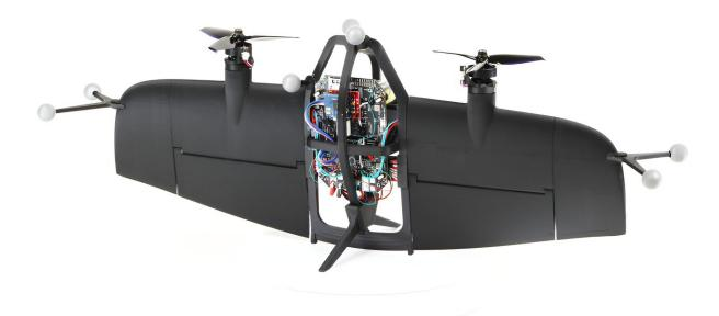
MIT researchers developed new algorithms for trajectory planning and control of fixed-wing "tailsitter" aircraft, which are faster and more efficient than traditional quadcopter drones. Credit: Massachusetts Institute of Technology
