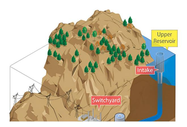
A closed-loop pumped hydropower system relies on an upper and lower reservoir. Credit: Al Hicks, NREL
