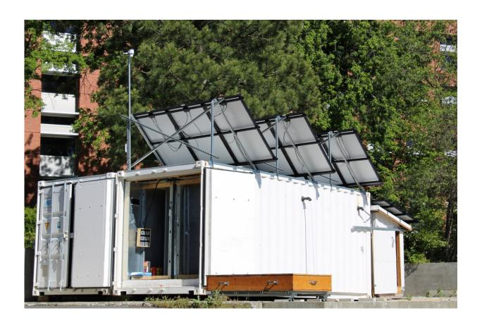
A 60 square-foot chamber inside a shipping container can test passive systems that use wind towers along with water evaporation instead of electricity to cool spaces. Credit: WSU
