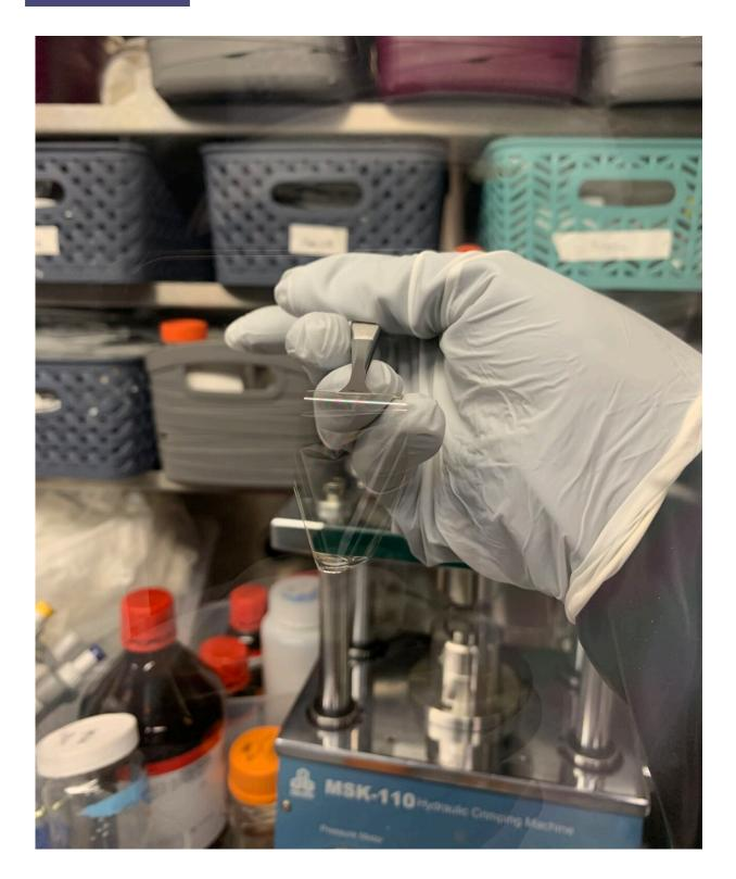
Photograph of the new transparent, thin-film FS-LiPON material which promotes a uniformly dense lithium metal electrochemical deposition under zero external pressure, with the aid of internal compressive stress and a gold seeding
