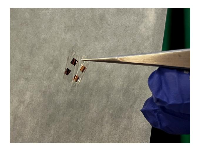
Photograph of the new transparent, thin-film FS-LiPON material which promotes a uniformly dense lithium metal electrochemical deposition under zero external pressure, with the aid of internal compressive stress and a gold seeding layer. The team also reports that this new stand-alone thin-film version of LiPON enables fundamental research (ss-NMR and Cryo-EM) of ion conduction and electrochemical performance. Credit: UC San Diego Laboratory for Energy
