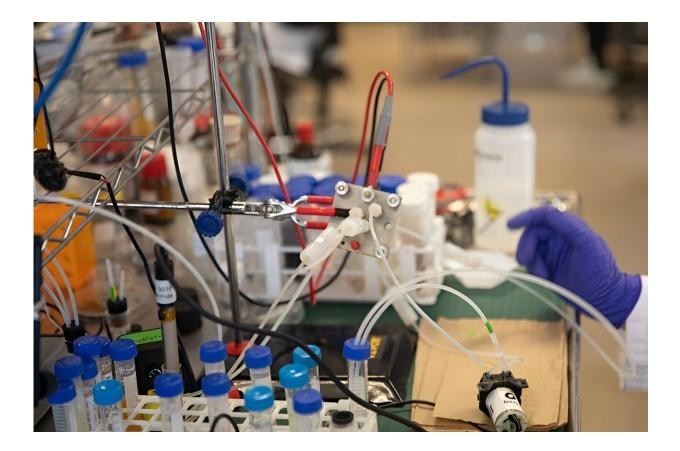
U of T Engineering researchers have created devices that can rapidly switch between electrolyzer mode and fuel-cell mode, increasing their overall efficiency at regenerating the liquid solutions needed for carbon capture. Credit: Tyler Irving
