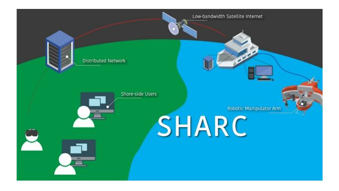
A new framework for oceanographic research provides a way for shore-based observation and control of robotic sampling processes. Credit: Phung, Billings, Daniele, Walter, Camilli
