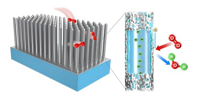
Vertically aligned coaxial nanowires in an electrode with protons transported in the ionomer core inside the nanowire. Electrons transported in the platinum nanofilm shell combine with oxygen to complete the fuel cell cathode reaction. Credit: Los Alamos National Laboratory
