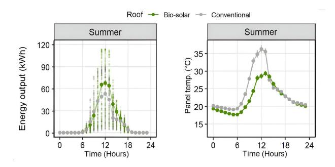
Energy output (left) and surface temperatures (right) of solar panels on a biosolar green roof and on a conventional roof. Credit: <u>Data: Green Roof & Solar Array –</u> <u>Comparative Research Project</u>
