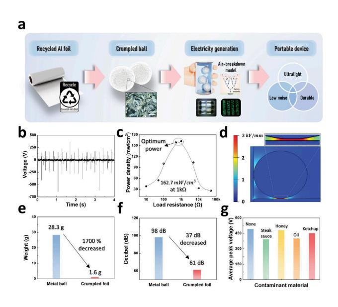
Concept and character of the RFCB-TENG. a) Schematic process diagram of a
