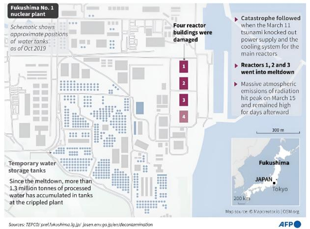
Graphic on the Fukushima nuclear disaster in 2011 and a schematic of the storage tanks for treated water at the power plant.
