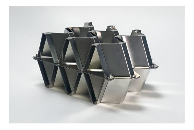
The MIT researchers modified a common origami crease pattern, known as a Miura-ori pattern, so the sharp points of the corrugated structure are transformed into facets. The facets, like those on a diamond, provide flat surfaces to which the plates can be attached more easily, with bolts or rivets. Credit: Massachusetts
