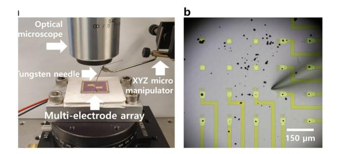
Particle & chip assembling process a) Experimental setup for particle positioning on a multielectrode array using an xyz micro-manipulator and optical microscope. b) Optical micrograph of the tungsten needle and randomly scattered particles during the particle positioning process. Credit: *Energy & Environmental Science* (2023). DOI: 10.1039/D3EE00953J
