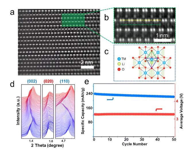
(a) HADDF-STEM image along the [110] zone axis. (b) The corresponding enlarged area to emphasize the atomic arrangement. (c) The schematic diagram of the honeycomb local structure pinned with TMLi ion. (d) The stacked peak profiles of the in situ XRD patterns. (e) Voltage and capacity stability at C/3 in
