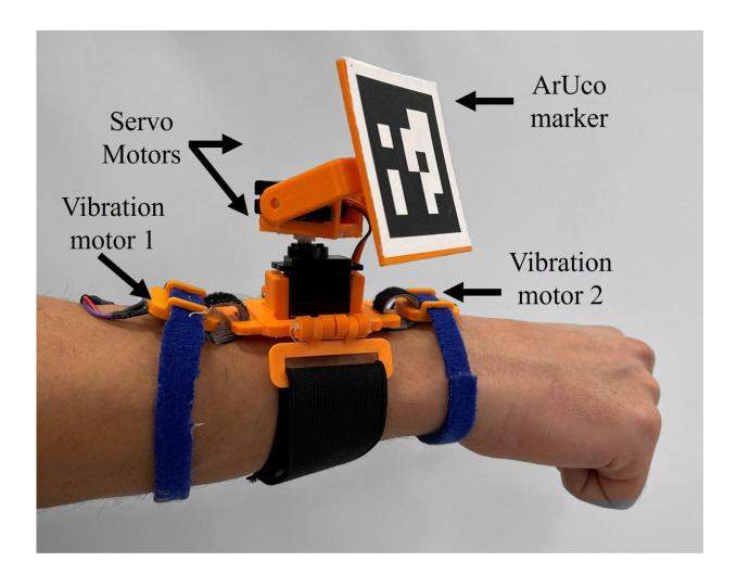
ArUcoGlide: a novel wearable robot for position tracking and haptic feedback. An ArUco marker is located at the end effector to adjust its orientation, and the two vibration motors provide haptic feedback to the user. Credit: Alabbas et al.
