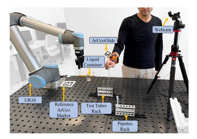
Real experiment using the ArUcoGlide system. The robot takes an empty pipette, fills it with liquid from the container, and returns it. The user counts liquid drops in a test tube. Credit: Alabbas et al.
