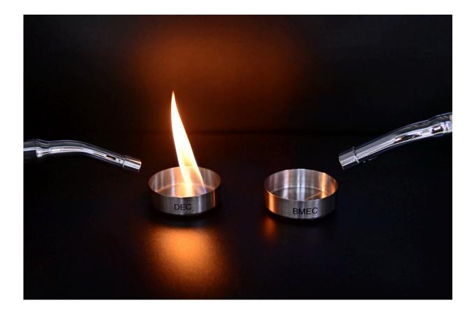
(Left) Electrolyte of a commercial lithium-ion battery (DEC) and a new electrolyte (BMEC) developed by a joint research team from KIST, KITECH, and KAIST (right). Credit: Korea Institute of Science and Technology
