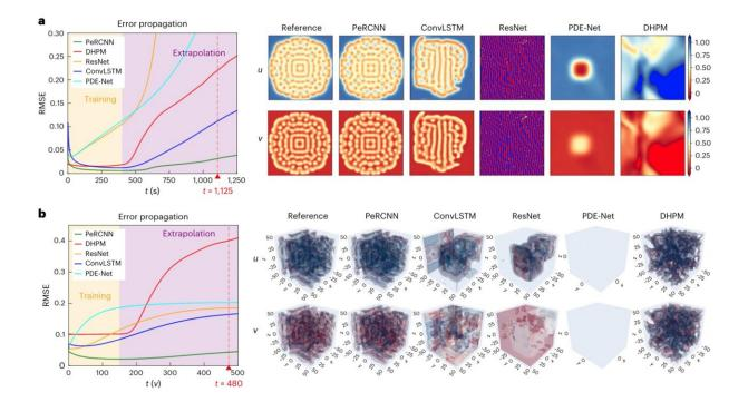
Error propagation curve of the prediction and the extrapolated snapshots from each data-driven model compared with the reference solution. Credit: UCAS
