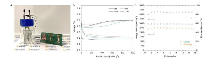
LCB pouch cell performance. (a) Photograph of the Pt-based LCB pouch cell lighting up the LED array. Discharge–charge curves (b) and energy density and energy efficiency versus cycle number profiles (c) of the Pt-based LCB pouch cell with a limiting capacity of 1000 mA h g<sup>-1</sup>. Credit: *Energy & Environmental Science* (2023). DOI: 10.1039/D3EE00794D
