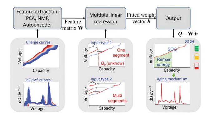
The workflow for predicting an entire charge curve of a battery based on a portion of the charge curve. Both a continuous segment and multiple separated segments can be used as the input. The output charge curve can derive many key states (SOC, SOH, and remaining energy) and even the aging mechanism of the battery using the dQ dV<sup>-1</sup> analysis. Credit: *Advanced Science* (2023). DOI: 10.1002/advs.202301737
