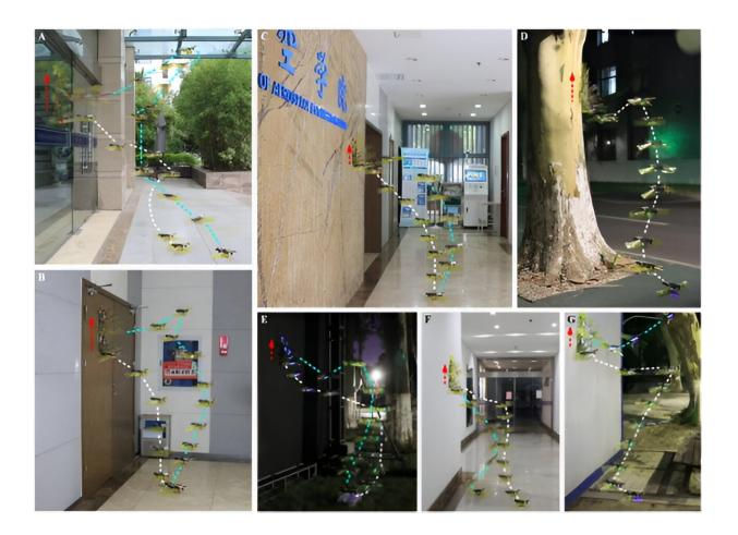
The robot landing, climbing, and taking off on a variety of vertical walls. Credit: *Research*
