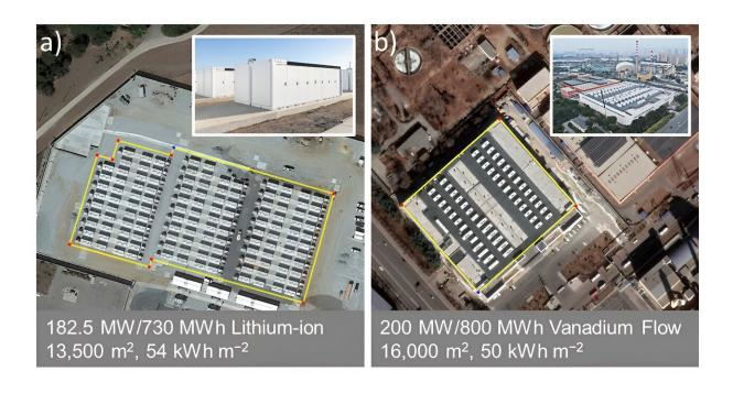
Satellite images and photos of some of the largest lithium-ion and vanadium flow batteries deployed to date. Credit: *Energy Advances* (2023). DOI: 10.1039/D3YA00208J
