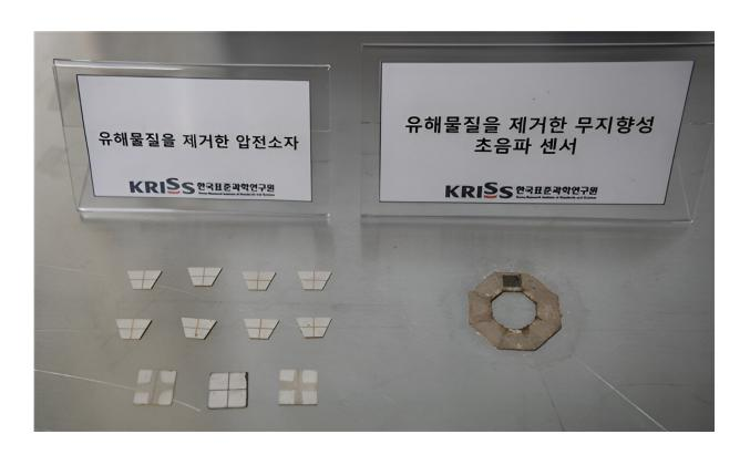
Segmented lead-free piezoelectric elements in shear wave mode (left) and the resulting omnidirectional sensor (right). Credit: Korea Research Institute of Standards and Science (KRISS)
