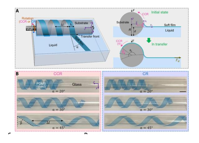
Elastocapillary rolling transfer weaves soft film to spatial helical structure on curved substrates. Credit: *Science Advances* (2023). DOI: 10.1126/sciadv.adh9232
