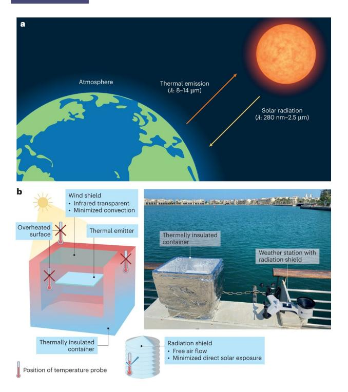
Electricity-free radiative cooling technology. a, A schematic illustration of the heat exchange channel, whereby objects on the ground can emit heat through an atmospheric window within the wavelength ( $\lambda$ ) range from 8 to 14 µm. b, A typical radiative cooling system operating in outdoor conditions, where the position of the probe used to monitor the ambient temperature is critical. Credit:
