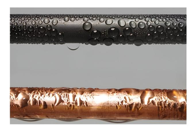
Copper steam condenser pipes coated with F-DLC (top) and without a coating (bottom). The F-DLC coating allows the condensed water to form into droplets rather than a thin film covering the pipe. Credit: The Grainger College of Engineering at the University of Illinois Urbana-Champaign
