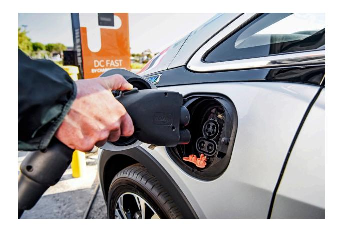
This photo provided by General Motors shows the combined charging system or CCS plug. It had been the dominant standard for EV charging until automakers decided to switch to Tesla's standard. Credit: Jessica Lynn Walker/Courtesy of General Motors via AP
