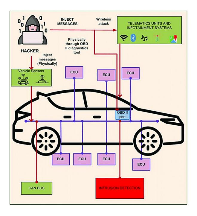
Your car has a computer network, and like most networks, it can be hacked. Electronic control units (ECUs) are sets of computer chips that control the various systems in your car. Credit: Khatri, Shrestha and Nam, CC BY
