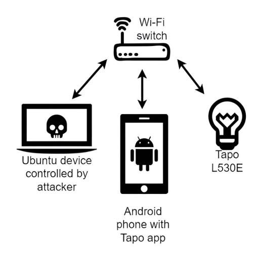
Setup B, network with a configured smart bulb. Credit: *arXiv* (2023). DOI: 10.48550/arxiv.2308.09019
