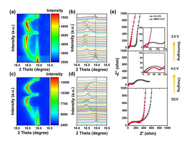
In situ XRD for D-LCO (a-b) and upcycled MNS-LCO (c-d); (e) EIS spectra. Credit: Liu Zhenzhen
