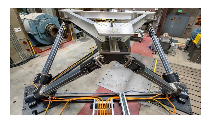
The lab's new large-amplitude motion platform, or LAMP, can mimic ocean motions, including waves up to 8 feet high, and supports devices weighing about as much as a small recreational vehicle. Credit: Bryan Bechtold, NREL
