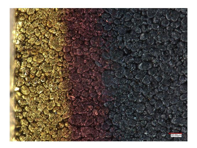
The distribution of lithium concentration indicated by colors during charging process of a graphite negative electrode. Credit: Queen Mary, University of London
