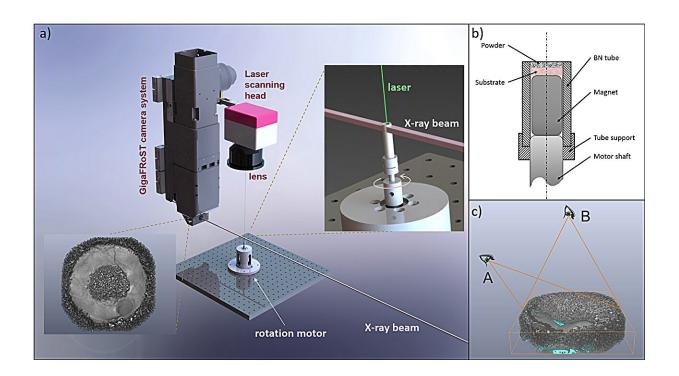
Setup for operando tomographic microscopy during LPBF of ceramics.. Credit: *Communications Materials* (2023). DOI: 10.1038/s43246-023-00401-3
