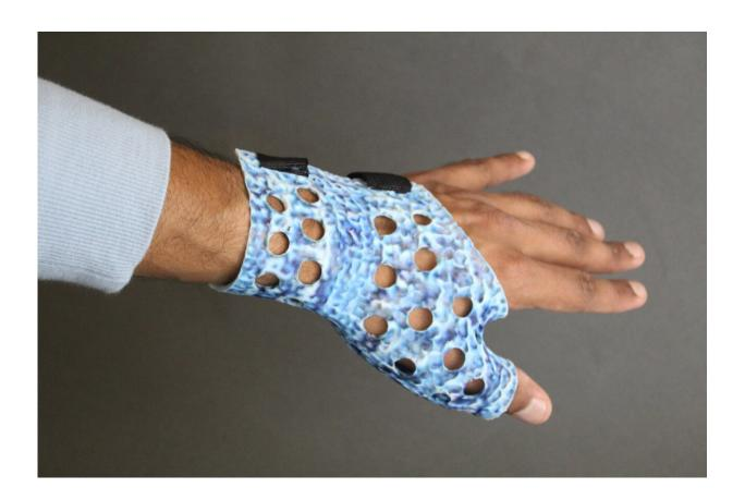
MIT researchers developed a user-friendly interface that enables a maker to customize the color, texture, and shape of the aesthetic characteristics of an open-source 3D model from an online repository, without affecting the functionality of the fabricated object. Credit: Faraz Faruqi and Stefanie Mueller
