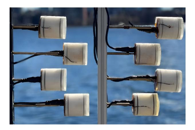
The device is an array of piezoelectric transducers that enables battery-free underwater communication. Credit: Massachusetts Institute of Technology
