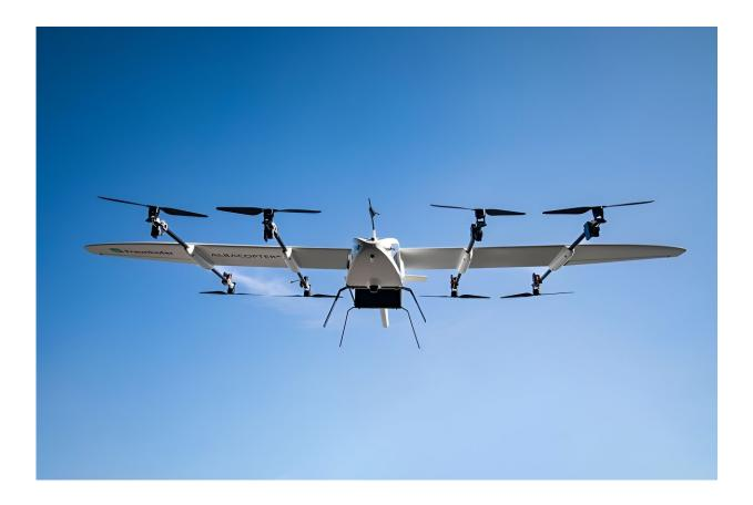
The ALBACOPTER—a cross between a multicopter and a glider. Credit: Fraunhofer IVI
