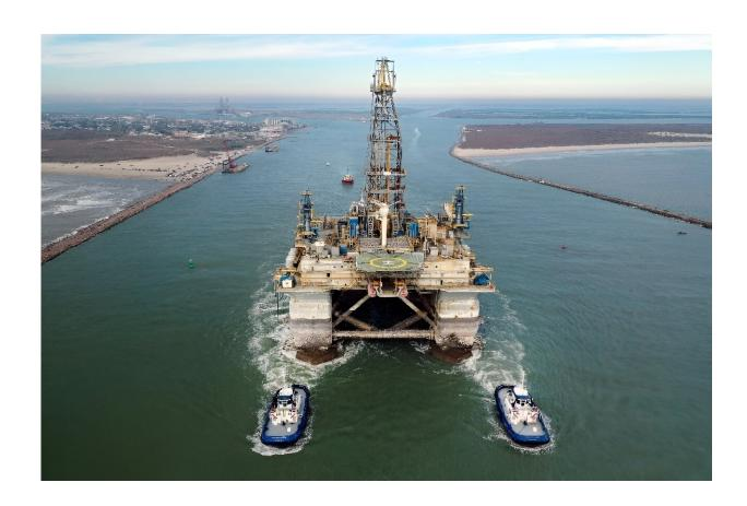
In this aerial image from a drone, tug boats tow the semi-submersible drilling platform Noble Danny Adkins through the Port Aransas Channel into the Gulf of Mexico.
