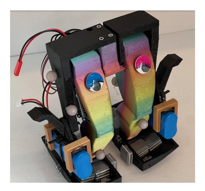
The "simplest" hip-actuated bipedal robot consisting of only two rigid bodies and
