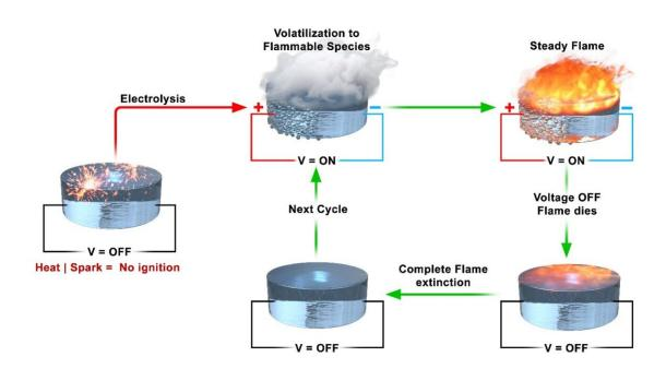
Process of inciting and stopping combustion with ionic liquid. Credit: Reprinted with permission from the American Chemical Society
