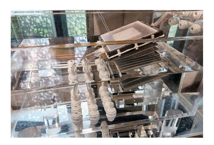
MIT researchers have designed a new solar desalination system that takes in saltwater and heats it with natural sunlight. The system flushes out accumulated salt, so replacement parts aren't needed often, meaning the system could potentially produce drinking water at a rate and price that is cheaper than tap water. Credit: Jintong Gao and Zhenyuan Xu
