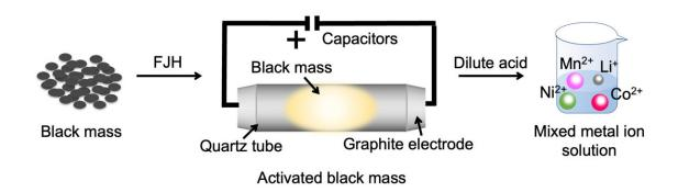
Schematic of the battery recycling process developed by Rice University scientists that uses their signature Joule-heating technique to remove the inert layer on battery metals and lower their oxidation state, making them soluble in low-concentration acid. Credit: Tour lab/Rice University
