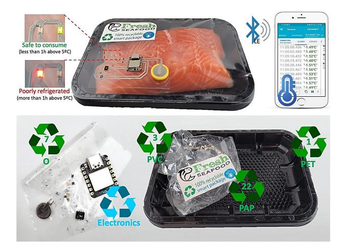
1) A printed smart label integrated in a package of perishable fresh food monitors its storage temperature over time and informs consumer through two LEDs whether the item is safe to consume or whether there is the risk of contamination due to poor refrigeration. 2) Both the food package and the integrated smart label can be fully recycled using conventional means and the
