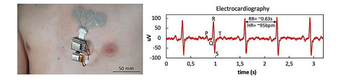
Electrophysiology patch adhered to the user'schest, over the sternal portion of the left pectoralis major muscle, connected to a biopotential recording system and battery. Credit: ISR - FCTUC
